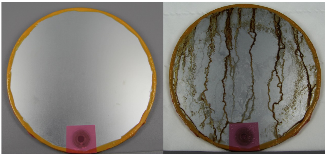
Figure 20: 3D4 (DC with 2 PR layers) before NSS exposure (left) and after 720 h exposure (right)
