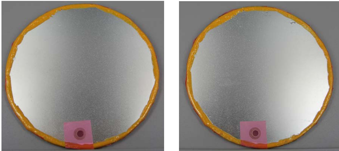
Figure 19: 5DB3 (DC with 2 PR layers) prior to exposure (left) and after 672 h NSS exposure (right)
