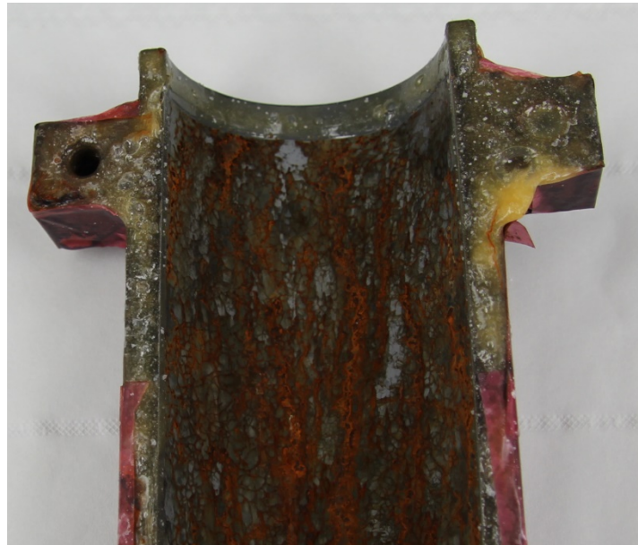
Figure 18: Zoomed image of 3F1 (PR plated) after 168 h exposure in NSS.
